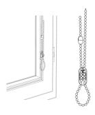
APPLY ONE HALF OF THE COUPLER TO EACH END OF THE CHAIN AND THEN LOCK BOTH COUPLER HALVES.
